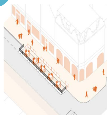
Temporary footway widening works: Type 2
