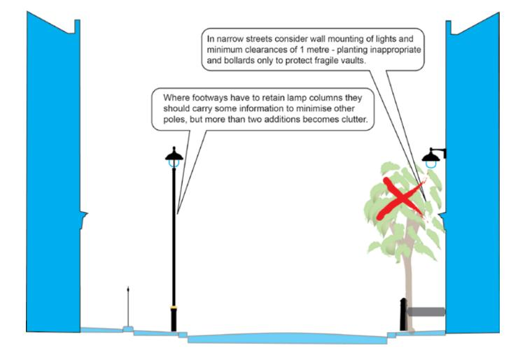
Above: diagram 5 showing typical placement regimes in a narrow street. Below: diagram 6 showing typical placement regime in a mews or alley.
