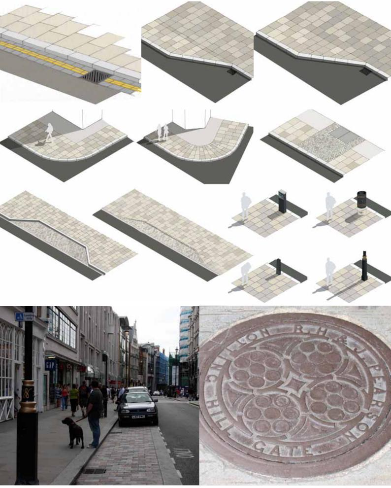
Top: diagrams showing principles for setting out paving slaps, kerb details and placement of key items with the type and bond expected throughout the city, more information is referenced in the Catalogue and through working details. Below: the theory in practice at Long Acre and a preserved coal-hole cover that adds character to some streets.
