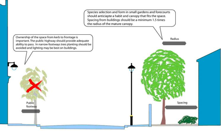
Spacing of items along the street: careful consideration needs to be made of the effects of trees on other items of street furniture and their functions. Interference with CCTV and the spread of lighting and radio waves means more a holistic approach to the overall placing of items is needed.
