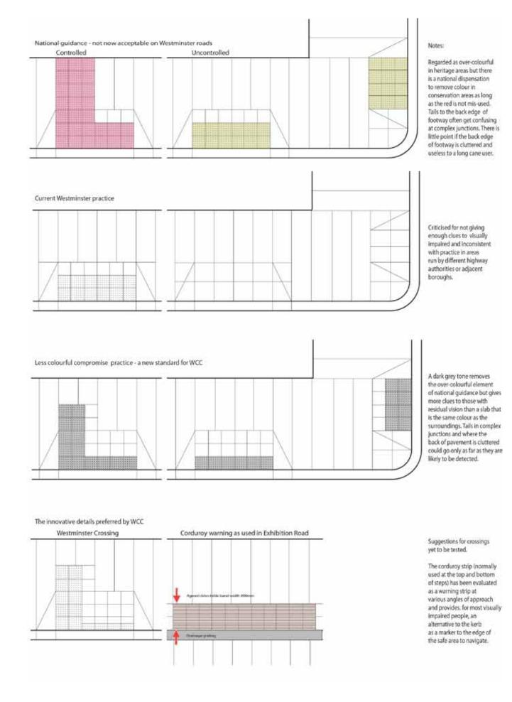
Figure 1 - comparative ways of installing tactile paving - some yet to be evaluated.
