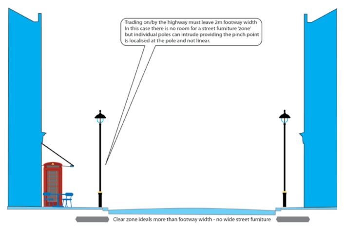
Above: diagram 7 showing typical placement regime in wider street. Below: diagram 8 showing typical placement regime in a boulevard and bus route.
