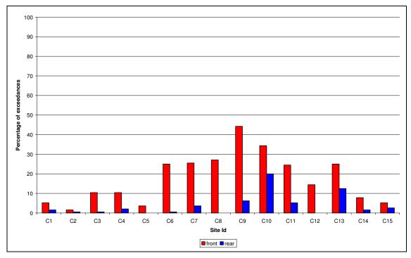
6.2.2 Both these graphs show that this level of 80 dB  $L_{AFmax,5min}$  is exceeded less frequently at the rear façade measurement position that at the front of the properties. However, at every property, this level is exceeded at some point during the day time at the front façade. In some cases, this value is exceeded during over 60% of the 5-minute time periods. At the
