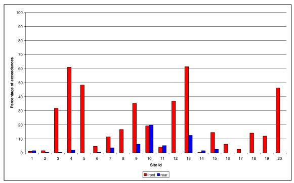
Figure 15. Percentage of day time 5-minute periods during which  $L_{\text{AFmax},5\text{min}}$  exceeds 80 dB(A) – Phase 2
