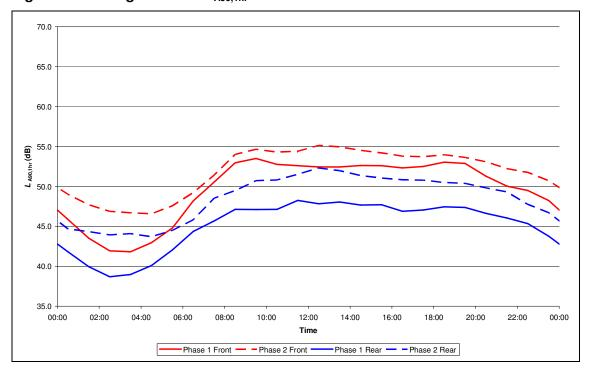
4.2.4 These graphs show the slight differences between the Phase 1 and Phase 2 average noise levels, with the difference generally being greater at the rear façades and for the  $L_{A90}$  noise indicator. It can also be seen that the difference is generally larger during the night time, with the average noise level dropping less at night over the Phase 2 sites than is seen for the Phase 1 sites. Again, this is clearest for the  $L_{A90}$  noise indicators.
