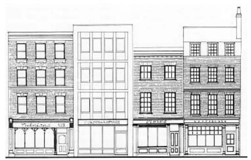
Architectural details, pilasters, entablature, mullions, panelled stallriser and door retained. In character with the façade and street.
