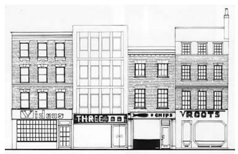
Inappropriate mock Georgian glazing, overlarge fascia and lettering. Removal of traditional features such as pilasters and entablature.
