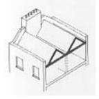
A double-pitched roof rests on three walls; the front and rear walls, and the load bearing spin separating the front and back rooms. The three walls run parallel to the two ridges of the roo
