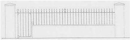
Typical elevation of domestic iron railings with brick piers on either side and brick dwarf wall.
