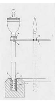
A FINIAL, drilled, screwed and spot welded to position.
