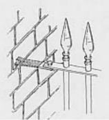
Example of fixing where the fish-tail end of the top rail can be built into the brickwork.
