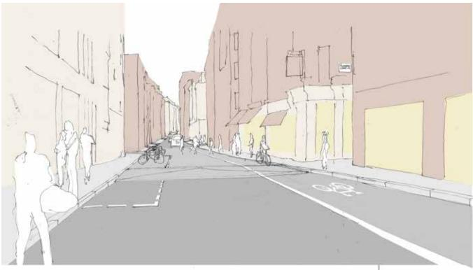
Looking north up Wardour Street showing the ideas for a dedicated cycle contraflow, flush carriageway in parts, parking and servicing kept to the west side of the street, improved paving surfaces and de-cluttering
