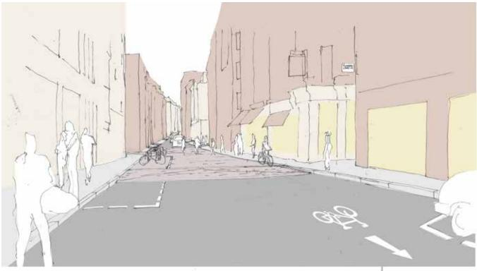
Looking north up Wardour Street showing the ideas for less delineated two-way cycling, raised tables, parking and servicing alternating between east and western sides, improved paving surfaces and de-cluttering
