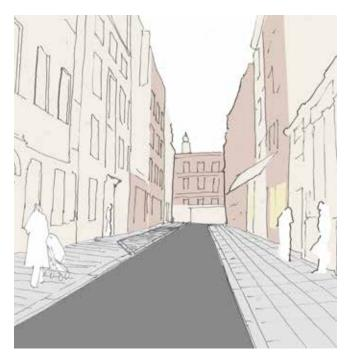
Archer Street: Widened pavement on north side with raised parking bays, de-cluttered and improved material condition.
