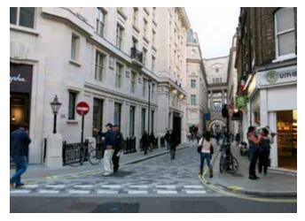
Air Street: repayed footways in EPS/York stone and granite kerbs, resurfaced carriageway raised at crossing points, payed with tricolour grey granite setts.
