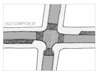
Idea 2: widened footways, raised parking/loading bays in dark granite setts, raised tables at junctions in granite setts.
