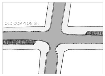
Idea 1: widened footways in concrete paving with raised parking / loading bays in dark granite setts, asphalt carriageways throughout.
