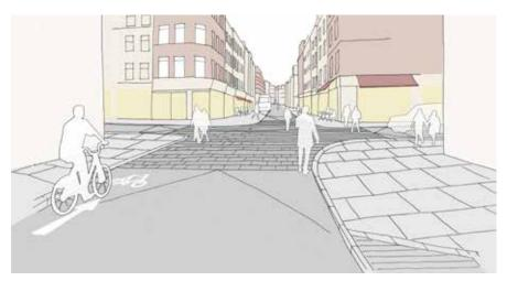
Idea 2: widened footways, raised parking/loading bays as above, with added granite setts to mark raised tables and flush kerbs at junctions.
