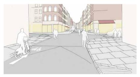
Idea 1: widened footways in concrete paving with raised parking/loading bays in dark granite setts.
