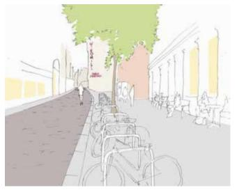
Great Windmill Street: new unified granite zone, widened pavement, decluttered, added cycle parking.
