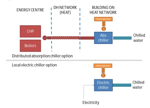
Figure 10-8 Schematic comparison of chilled water provision
