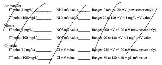
Record the following diagnostic numbers after calibration, by viewing the .glp file and reading the values for the day's calibration
