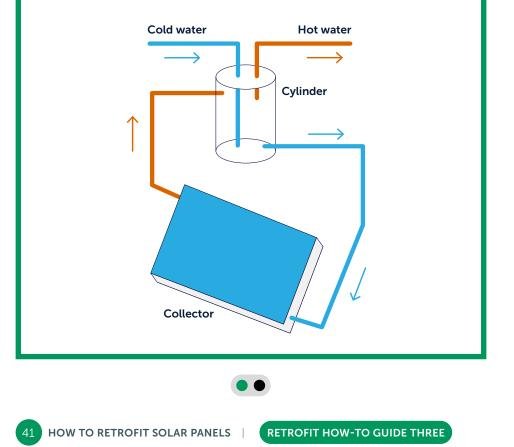
In the U.K. most of the solar thermal domestic hot water systems are based on indirect exchange and mechanical circulation.
