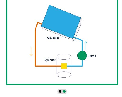
In the U.K. most of the solar thermal domestic hot water systems are based on indirect exchange and mechanical circulation.
