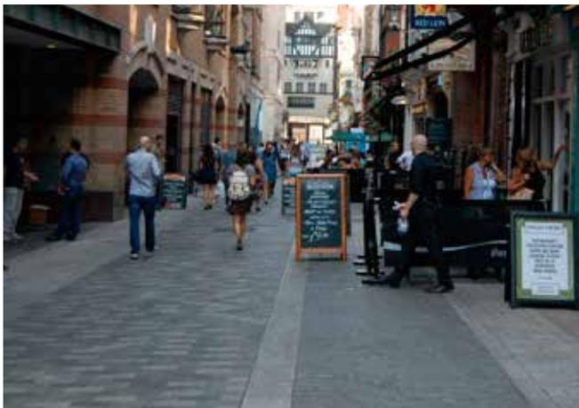
Kingly Street: resurfaced, raised carriageway and loading bays, paved with tricolour grey granite setts.
