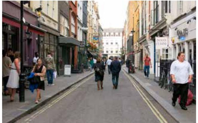
Typical condition in Soho: asphalt carriageways with granite kerbstones and concrete or asphalt footways on Bateman Street.
