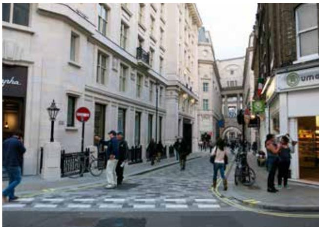
Air Street: repaved footways in EPS/York stone and granite kerbs, resurfaced carriageway raised at crossing points, paved with tricolour grey granite setts.
