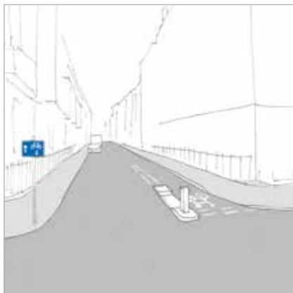
Some limited built elements: road markings and signage at entrances to one-way streets will indicate to vehicles to expect oncoming cyclists. A small traffic island could be installed for added protection.
