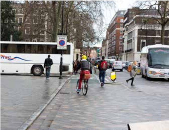
Byng Place, London Borough of Camden: a transition from a marked and segregated cycle lane to a wider space shared between pedestrians and cycles slows cyclists down.
