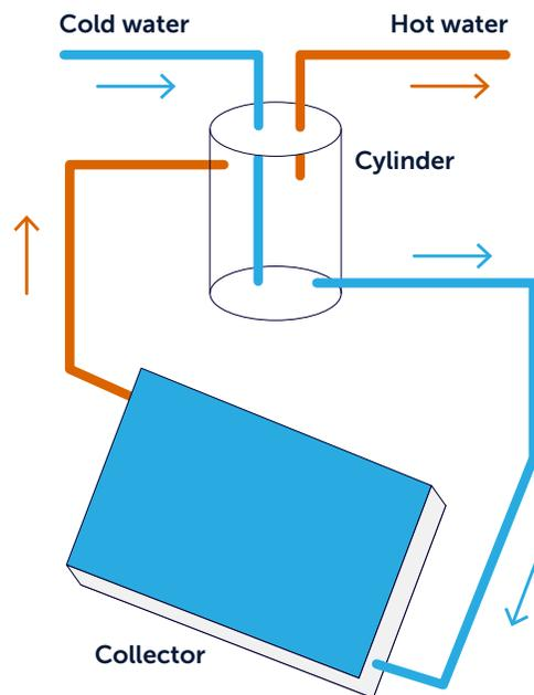
In the U.K. most of the solar thermal domestic hot water systems are based on indirect exchange and mechanical circulation.
