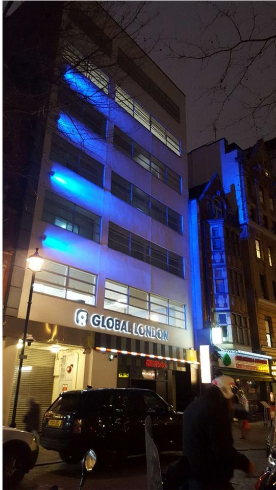
*Poor lighting design with excessive spill light*
