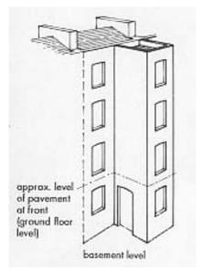
Fig. 7.3: Full height rear extension with flat roof.
