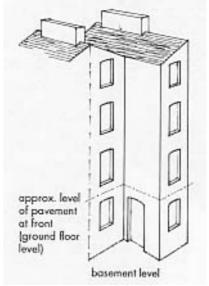
Fig. 7.4: Full height rear extension with pitched (valley) roof.
