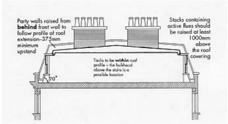
Fig. 11: Preferred section of flat-topped mansard roof. Scale 1:150.
