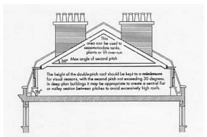
Fig. 12: Preferred section of double-pitched mansard roof. Scale 1:150.
