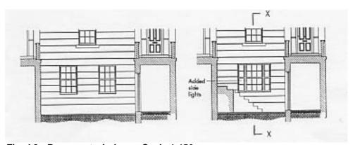
Fig. 4.2: Basement windows. Scale 1:150
