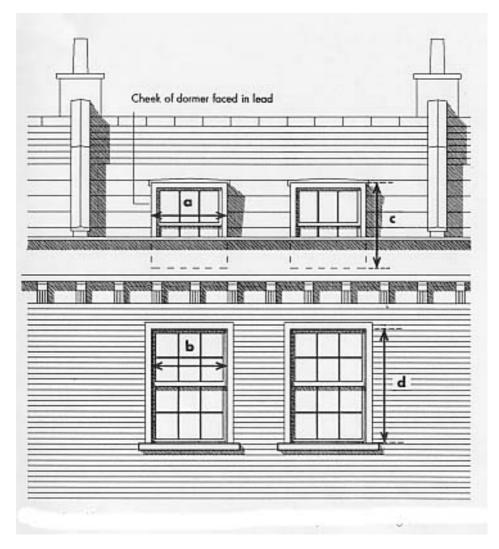
Overall width 'a' not to exceed opening width 'b' and height 'c' not to be greater than 'd'.
