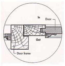
Fig. 2.3: Detail A (see section XX). Scale 1:5
