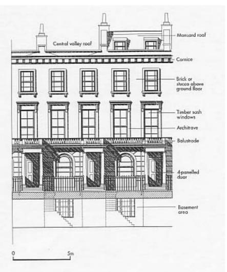
Fig. 1.2 (right): Front elevation of typical houses (Alderney Street). Scale 1:100.
