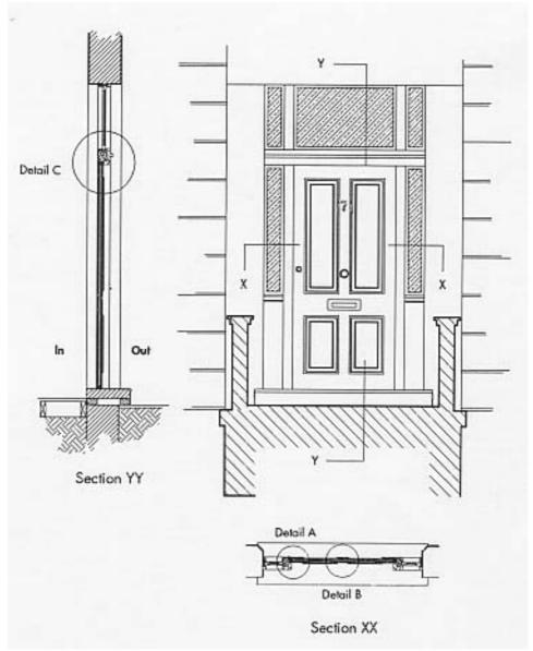
Fig. 2.1: Front door elevation and sections. Scale 1:40 (see also Details A, B C)
