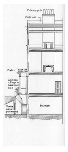
Fig. 1.1: Section through front of a typical Pimlico house.
