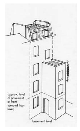
Fig. 8.1: Two storeys added to rear extension where original building has four storeys and basement.
