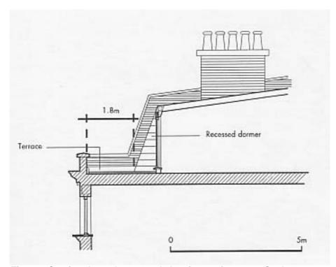
Fig. 15: Section through mansard showing roof terrace. Scale 1:100.
