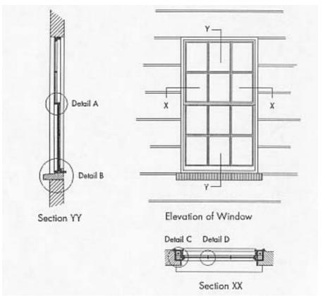
Fig. 3.1: Front windows - elevation and sections. Scale 1:40 (see also Details A, B, C, D)
